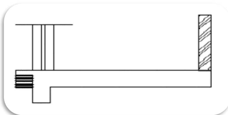
Figure III.16: porte-à-faux extérieur (balcon)
