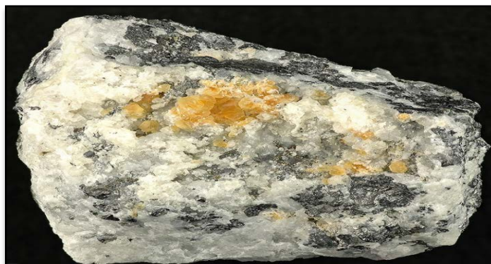
Figure I.1: Hydrotalcite ( Mg_6Al_2CO_3(OH)_{16} \cdot 4H_2O ).
