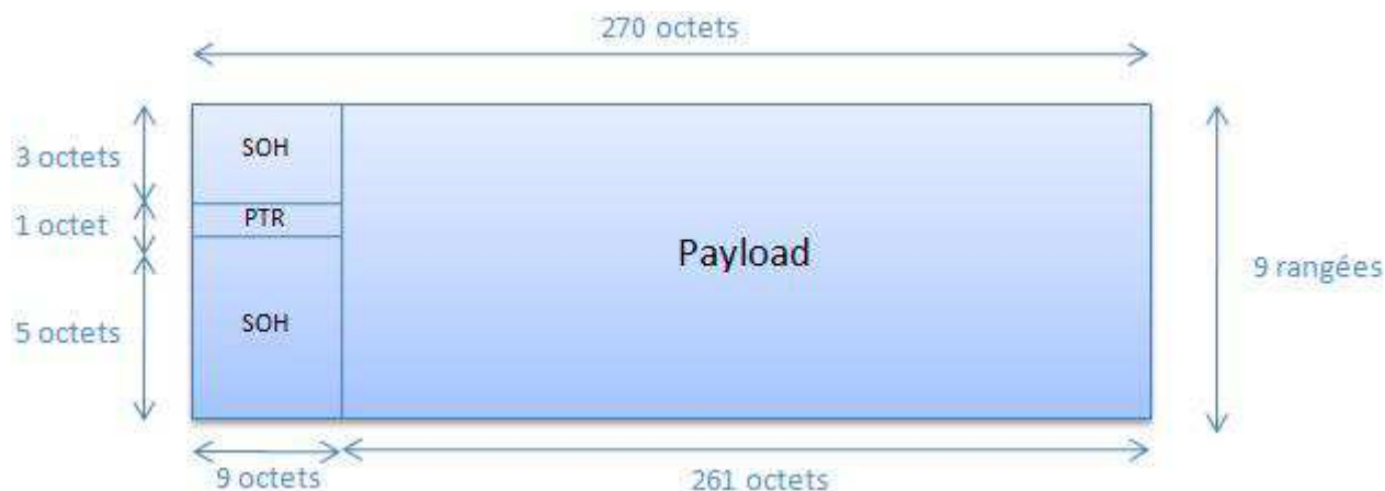
Figure II.2: Structure de la trame SDH STM-1
