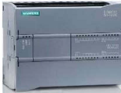
Figure II.6 : unité centrale CPU 1214C.
