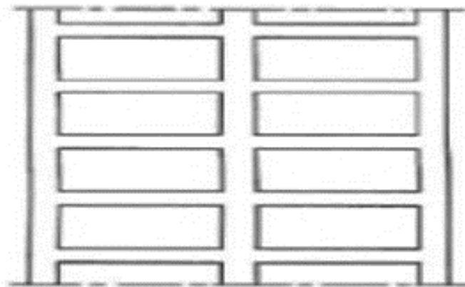
Figure I-12: ossature en portique [3]
