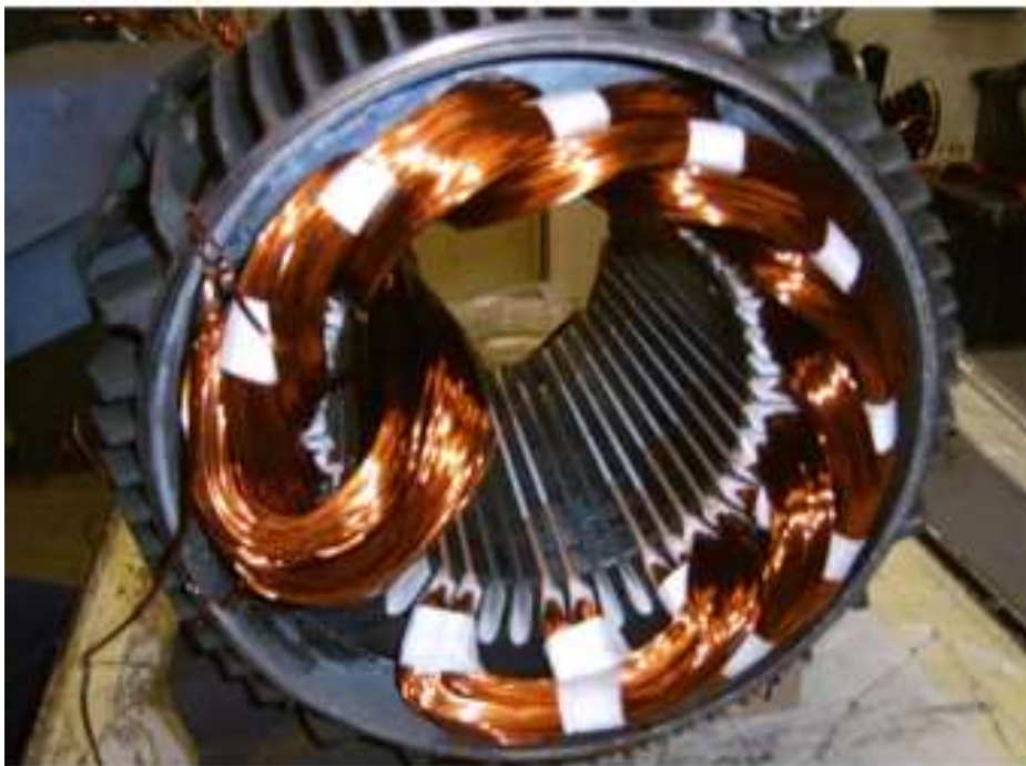
Figure I.3. Stator de la machine asynchrone [9]
