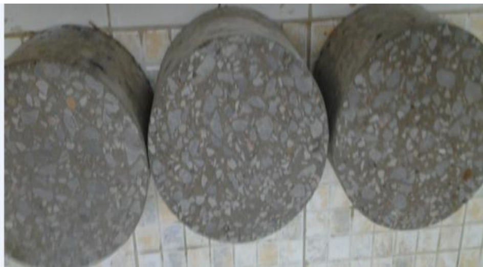
fig.6. Observation of the distribution of aggregates for the self-placing concrete
