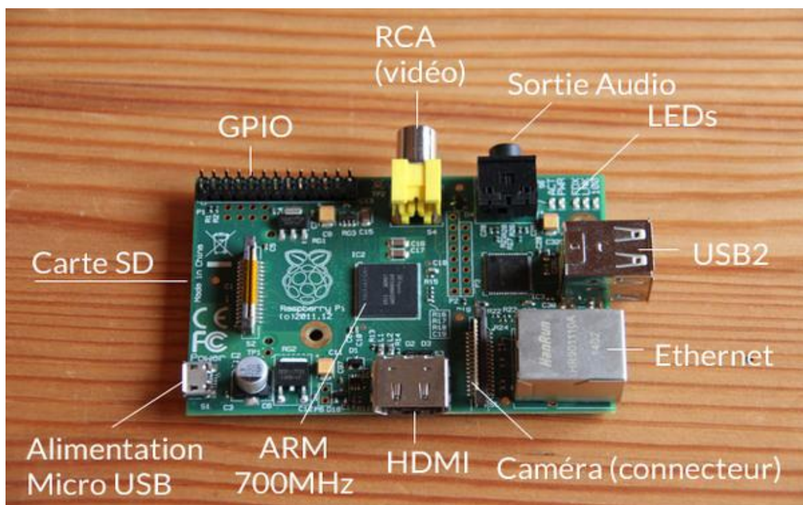
Figure 23: Composant de Raspberry pi.
