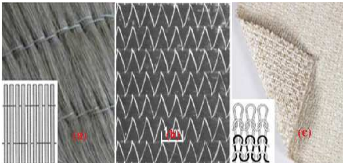
Figure I.10 : Renforts bidimensionnels non tissés:UD (a), NFC (b), tricot (c).
