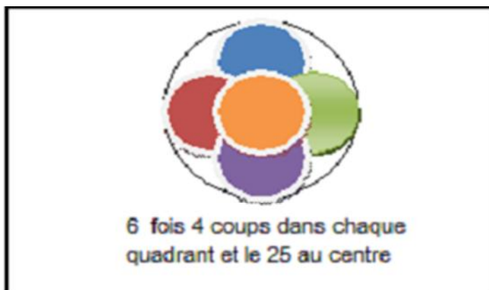
Figure III.13: Compactage des couches.
