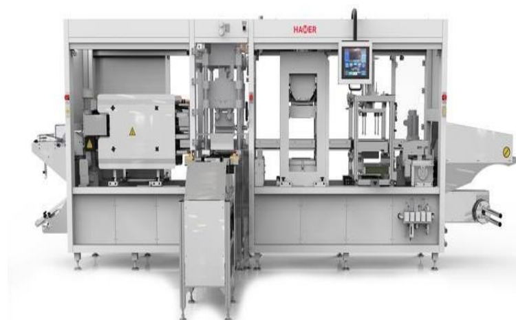
Figure 79: Automated aligner-forming system
