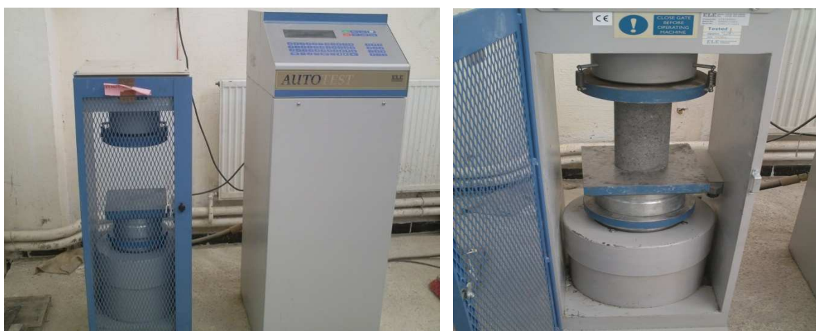
Figure III.B.5: Eprouvette en compression simple
