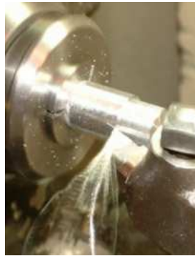
Figure VI.6: usinage de la surface extérieur de support-stator.
