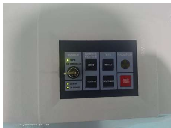
FIGURE 3.16 – Verrouillages de la clé " On "
