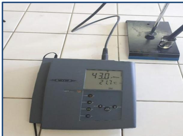
**Figure 13 :** Conductimètre (Inolab cond 720 wtw series)
