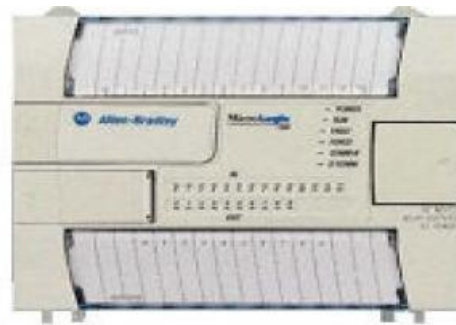
Figure IV-1 : Automate programmable de type compact (Allen-Bradley)
