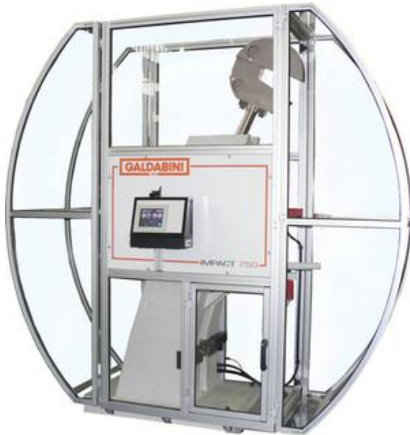
Figure II.4 : Mouton-pendule IMPACT 150 – 750 joules
