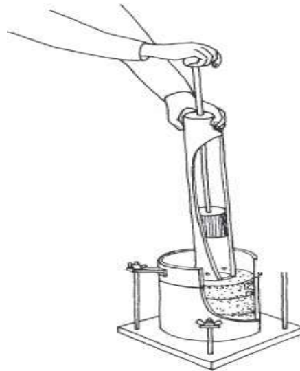
Figure IV.7 : Essai de compactage.
