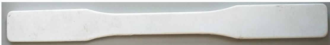
Figure III- 4: Epreuve axiale de norme (ASTM D-790) en HIPS.
