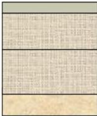
Figure I.2: Chaussées souples assise non traitée
