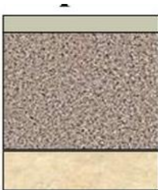
Figure I.2: Chaussées souples assise non traitée
