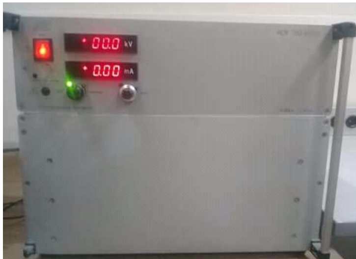
Figure III.8. Source de tension continue
