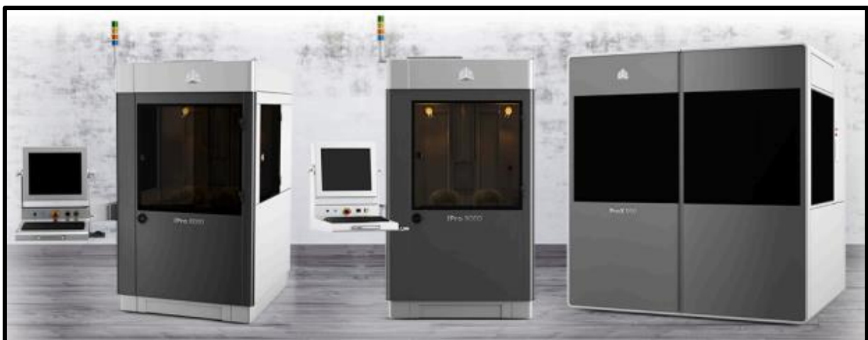
Figure III.4: Imprimante 3D SLA [5].
