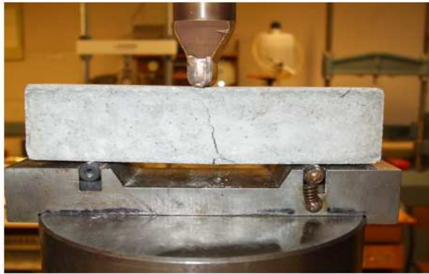
Figure 3.4: Essai de flexion 3 points.
