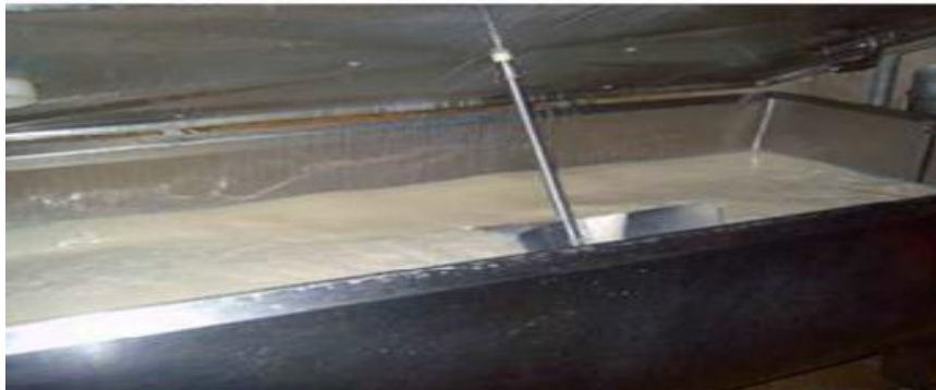
Figure 5: Cuve de coagulation
