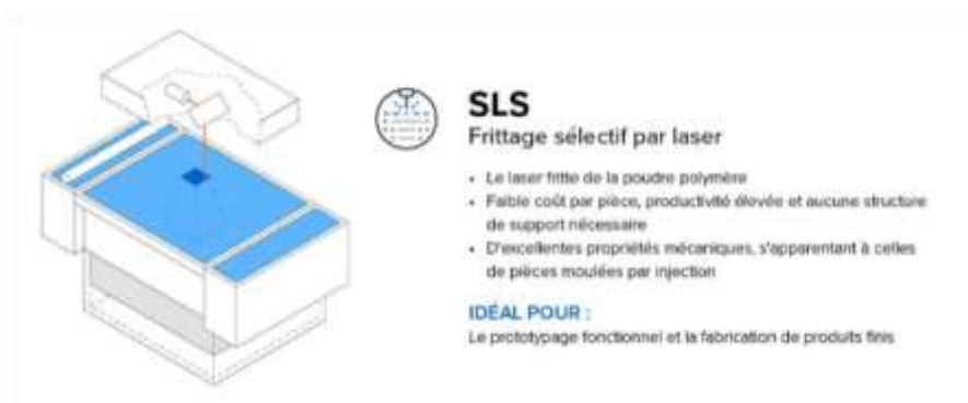
Figure 46: schéma d'une imprimante SLS (source : formlabs) [50].
