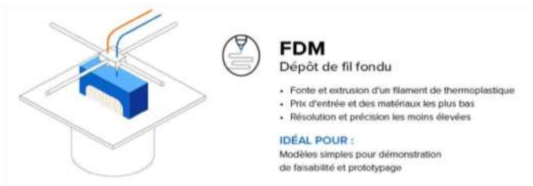
Figure 49: schéma d'une imprimante FDM (source: formlabs) [2].
