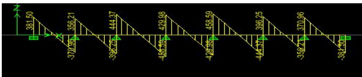
Figure XI.6 diagramme des efforts tranchants(ELU)
