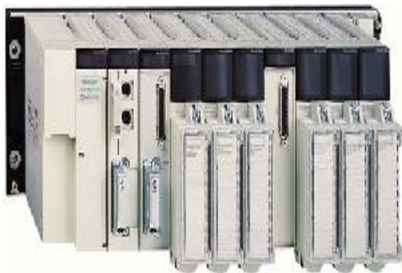
Figure II.4:Automate modulaire (Modicon).
