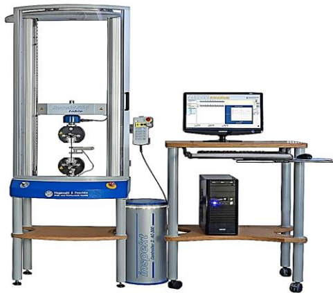
Figure III.16 : Machine de traction (Wikipedia)
