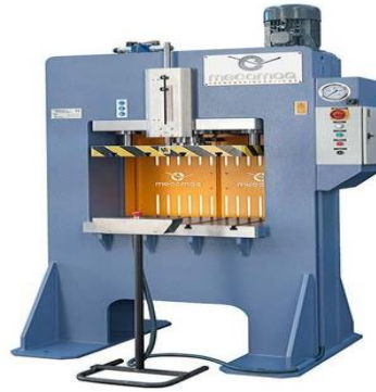
Figure III.4: Presse à arcade
