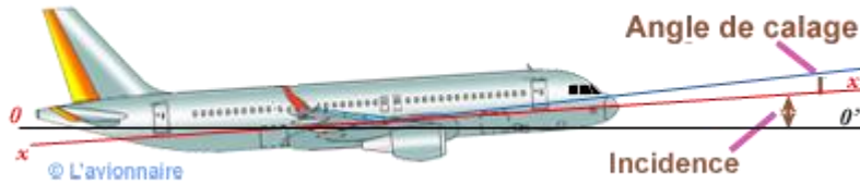
Figure 48 _ angle de calage [8]
