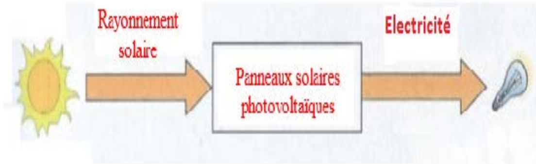
Figure II.3 : Effet photovoltaïque (PV).
