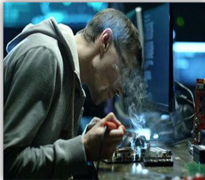
Figure II.43 : Le brassage tendre
