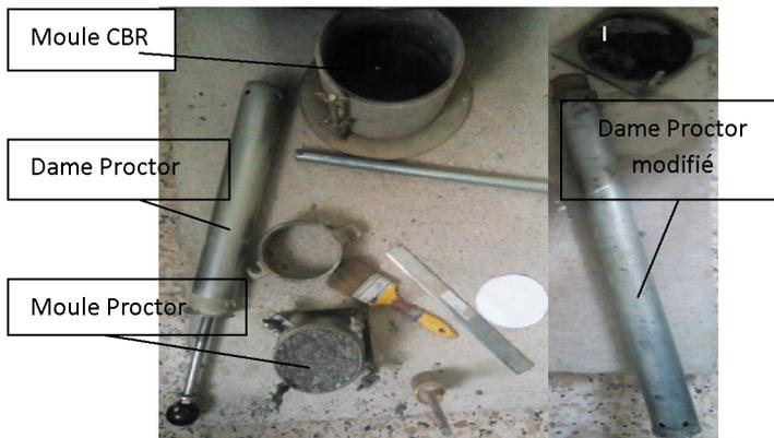
Figure II.2 : Appareillages Proctor [moule (PM, GM), dames de compactage (P Dame, G dame)].
