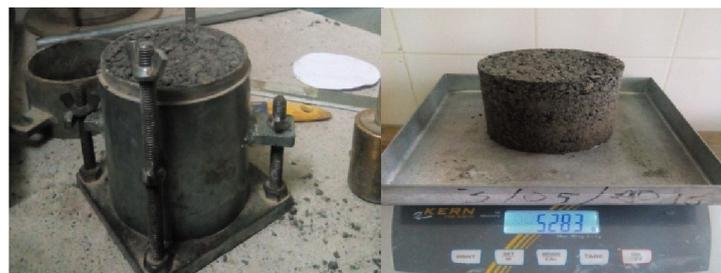
Figure IV.3 : Essai Proctor normal (grand moule).
