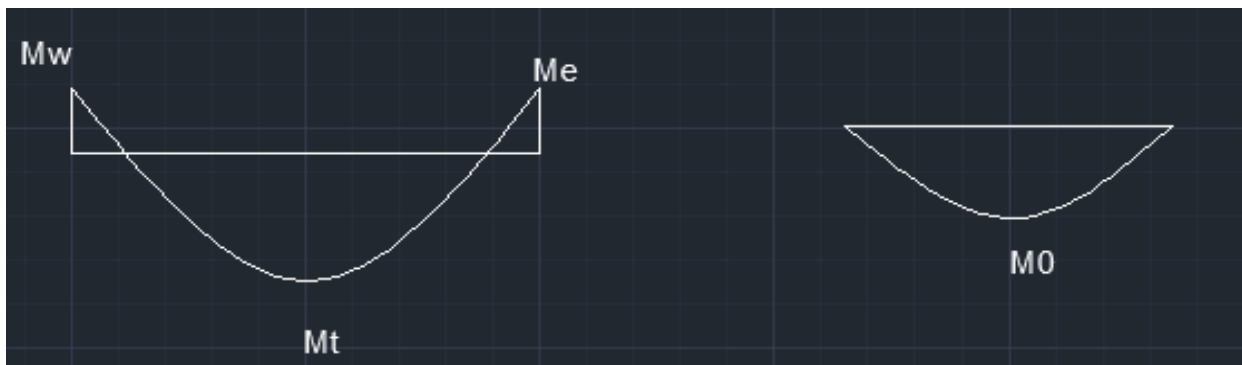
Figure III.3.4 Diagramme des moments.
