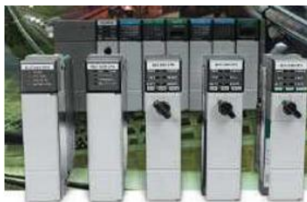
Figure III.5: SLC 500 Allen Bradley.
