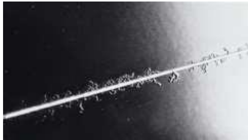
Figure I.7 Schéma illustrant la corrosion filiforme
