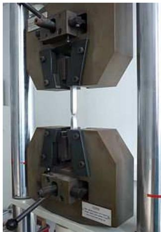
Figure. II.1 machine de traction
