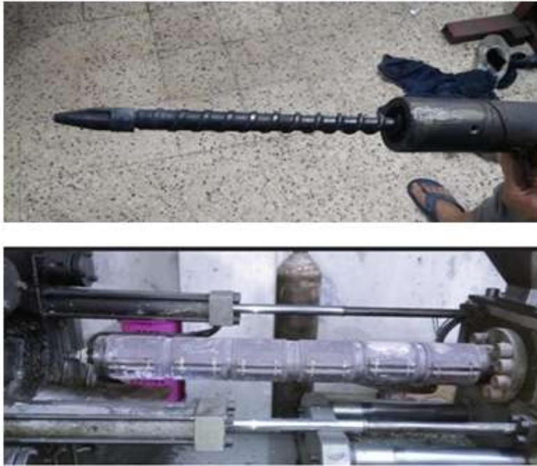
Figure V 8 station chauffage et la vis
