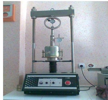
Figure III.11 : Appareil C.B.R.
