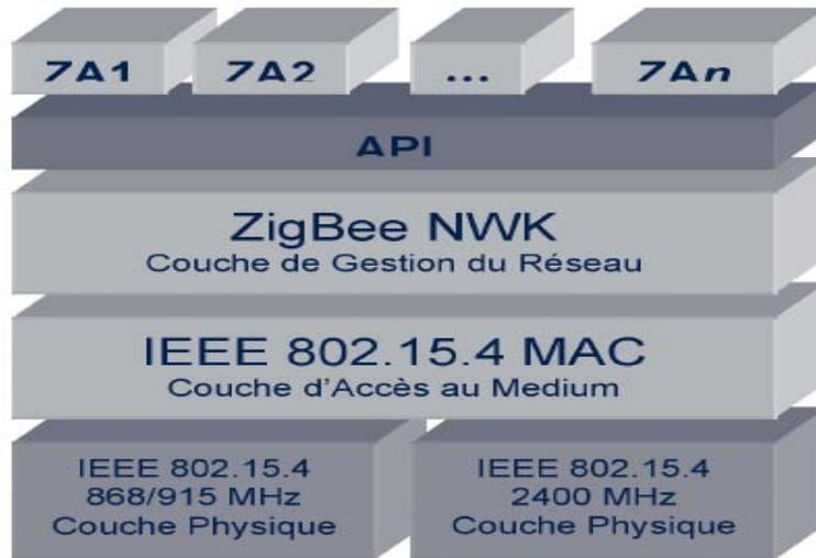
Figure I. 5. Pile protocolaire ZigBee
