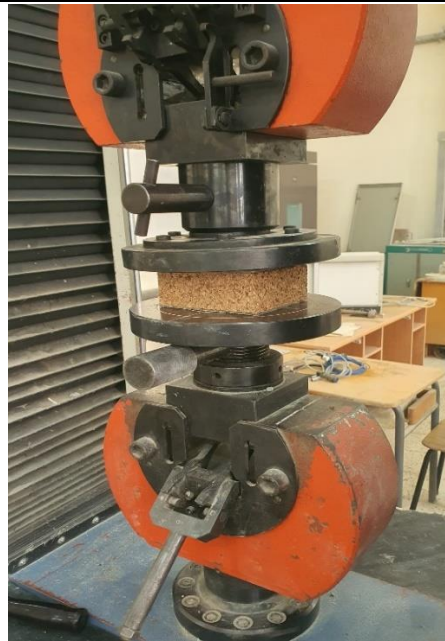
Figure II. 17: Essai de compression perpendiculaire
