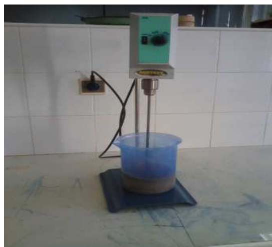
Figure -III.13 - : La dispersion de la suspension.
