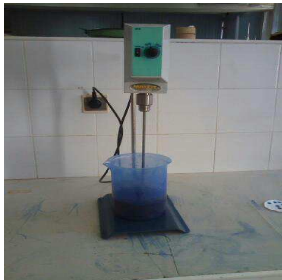
Figure -III.15 - : Le dosage de la suspension.
