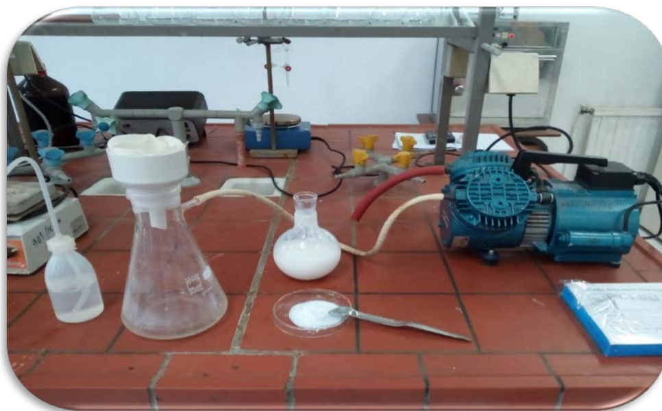
Figure II. 3: Filtration et lavage.
