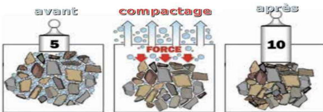
Figure IV.1. Compactage des sols.
