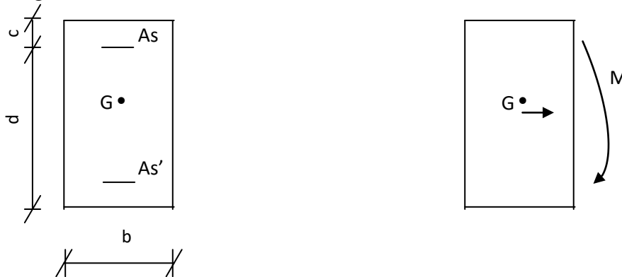
Figure III.3.2: section de balcon.
