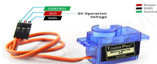
Figure II.27: Brochage de servomoteur SG-90.
