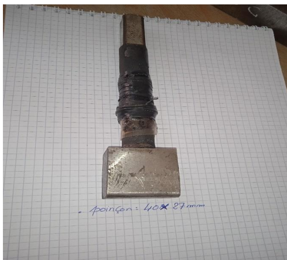
Figure II.7 dimension du poinçon 40 x 27mm
