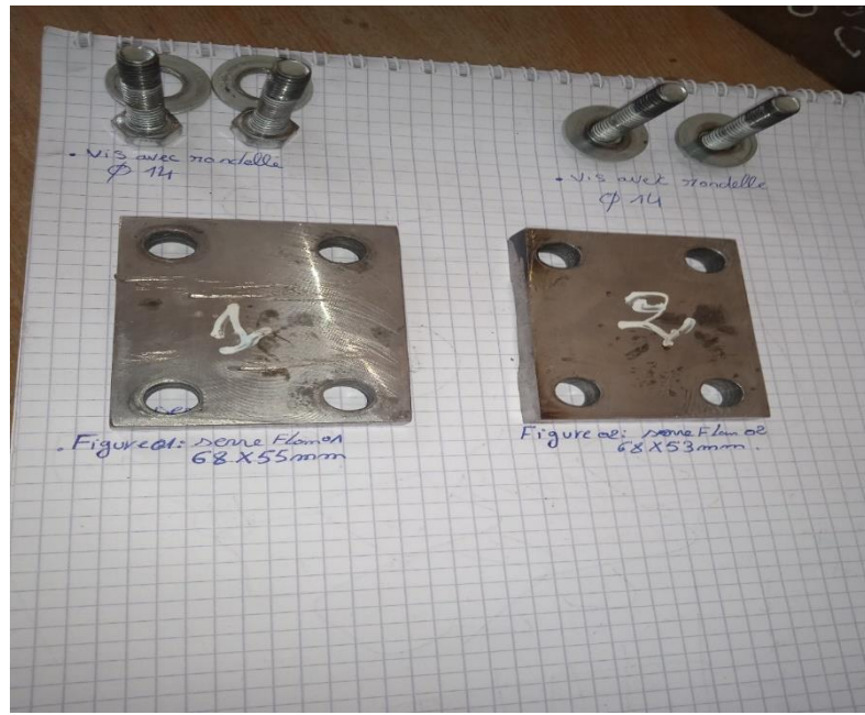
Figure II.6 les dimensions de serre flan, (68 x55mm).
