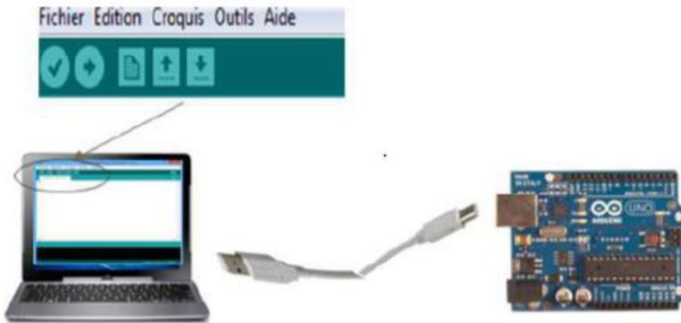
Figure II.14 : Communication carte Arduino et PC.
