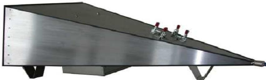
**Figure II-10:** cellule GTEM
