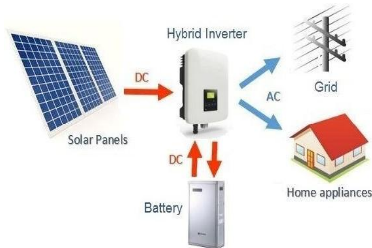
Figure 2.10 : Installation PV hybride [16].
